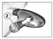
Turn bulb 2 clockwise to install. it in the bulb housing.
